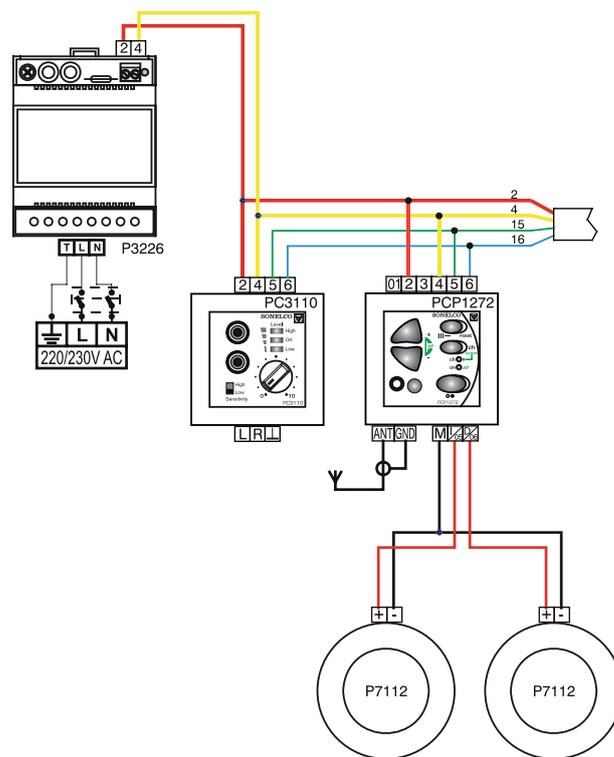
**FIGURE 3. INSTALLATION AS AUXILIARY POWER SUPPLY**
