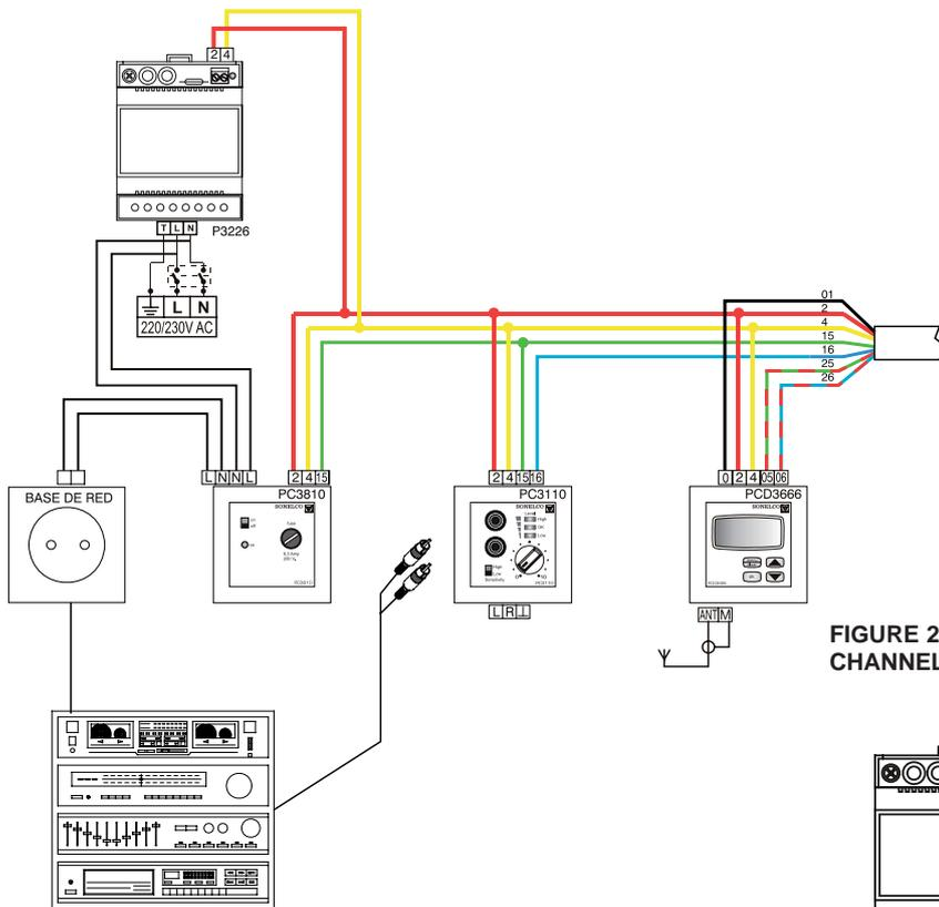
**FIGURE 2. CENTRALISED INSTALLATION WITH 1 STEREO CHANNEL CONTROL/PCP1272 LOCAL TUNER CONNECTION.**
